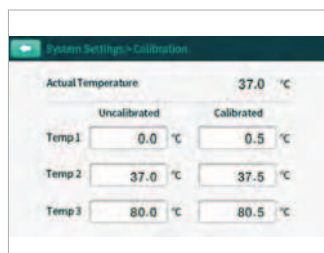
Accurate temperature control with 3-point calibration
