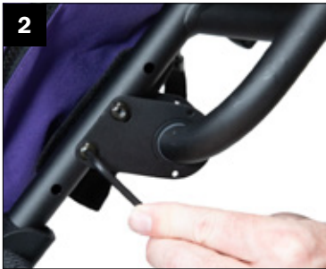
2. Use a 5/32" Allen key to move the placement of the bolt and armrest hardware up and down on the back frame tubes.
