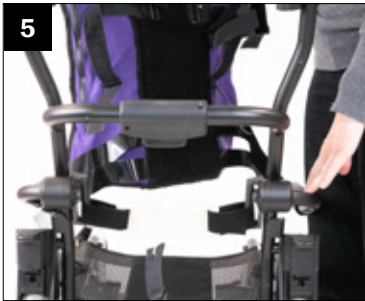
5. To remove the back upholstery, remove the hook and loop straps that attach the back upholstery to the frame, and take off upholstery.
