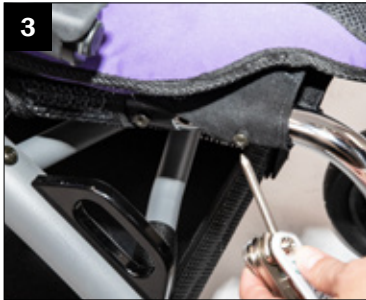
3. Remove the screws using a Phillips screwdriver, which attach the seat upholstery to the front riggings.
