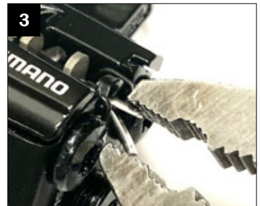
3. Remove cotter pin with pliers.
