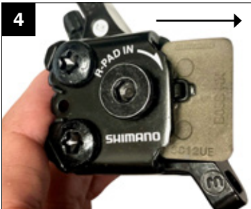
4. To remove pads, push pads through caliper.
