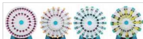
Tube holder set with disk (1.5ml / 5ml / 15ml / 50ml)
