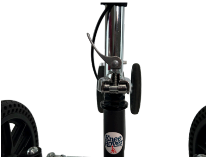
Raise the Quick Release Lever into the “U” shaped slot
