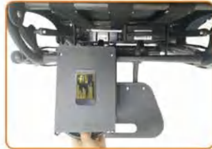
Photo 11. Installing the battery
