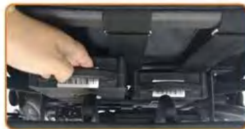
Photo 12. Removing the battery
