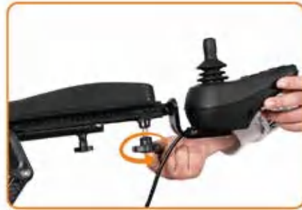
Photo 9. Secure joystick controller knob
